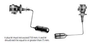
Table 16. Dimensions V and W with Minimum SG for Vertically-mounted Switches (Land Applications)
